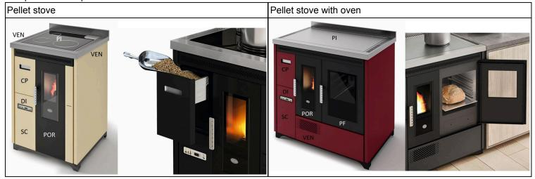
Key: VEN: ventilation air outlet; PI: Upper plate in steel or ceramic glass (only version without oven); CP: extractable pellet drawer; DI: display; POR: firebox door; PF: oven door; SC: lower door (location of ON/OFF switch, safety thermostat, RS232 socket).
