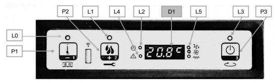
The control board can be managed by simply pressing a few buttons on the control panel. A display and the LED indicators inform about the stove operational status. When in programming mode all the parameters that can be modified using the buttons are shown on the display.
